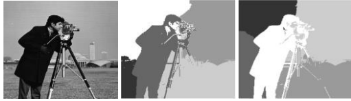
Fig. 8. Left to right: Cameraman: 256 by 256 8-bit grayscale image, floating-point segmentation and fixed-point segmentation result.
