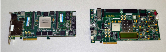
Fig. 3. Development boards: Terasic DE5-Net (left) and Xilinx KC705 (right).
