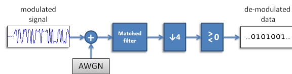
Fig. 1. Diagram of a simple binary phase-shift keying (BPSK) receiver circuit with additive white Gaussian noise (AWGN).
