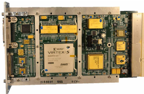
Fig. 6. NASA GSFC SpaceCube 2.0 flight computer (courtesy: NASA GSFC).
