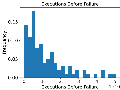
Fig. 4. Execution time before first failure for experiment one in subsection VI-B (target probability of failure: 10^{-9} ).
