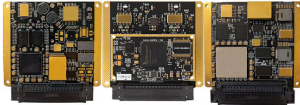
Figure 1: CSP Rev. C FM (Left), \mu CSP Smart Module (Middle), and SSP FM (Right)
