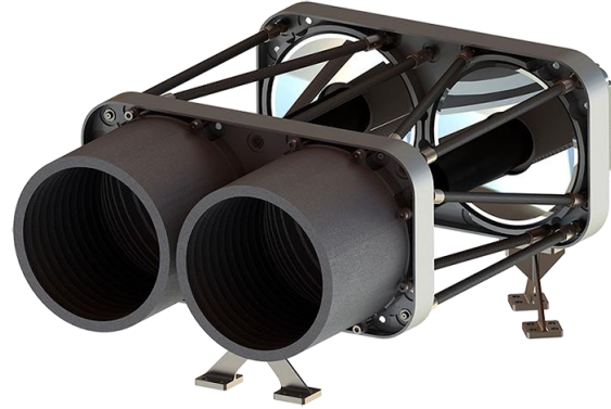
Figure 5: SATLANTIS iSIM-90 Opto-Mechanical Structure
